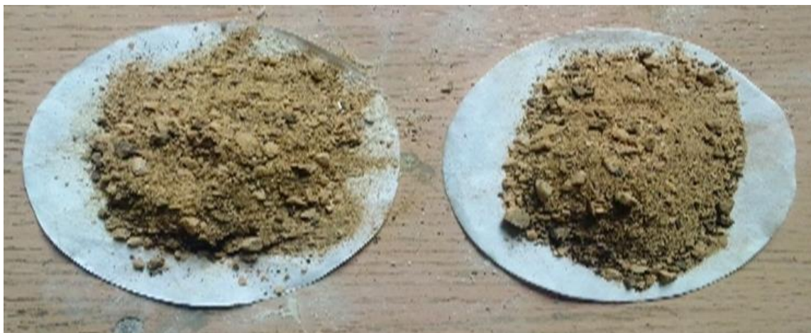
Figure 2. Pulverized sample of baryte from Azara
